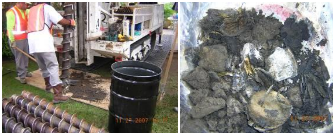
Figure 29: Drilling Exploration in Backyard of Residence to Define Southern Extent of Former Landfill; Waste Fill Material from Boring
