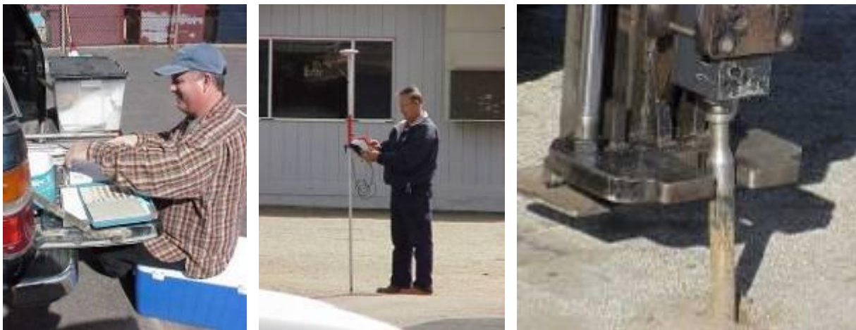
Figure 43: Geologist documents direct push boring observations in boring logs. Location of borings is surveyed using GPS surveying equipment. The direct push sampler has a diameter of 1.5 inches.
