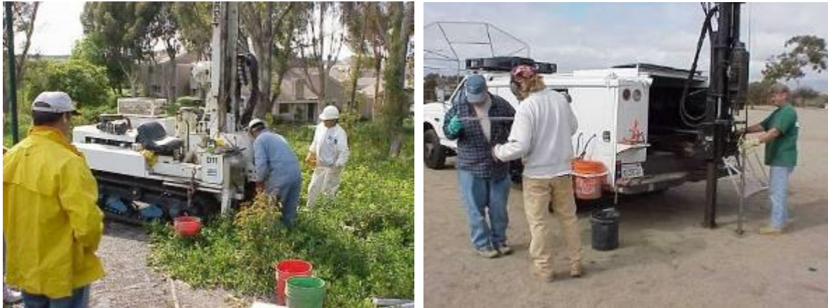
Figure 16: Direct Push Exploration and Sampling Methods (push core sampler into geologic strata)—Investigation disturbance is a nominal 2-inch diameter hole (important consideration in developed areas with dense subsurface utilities)
