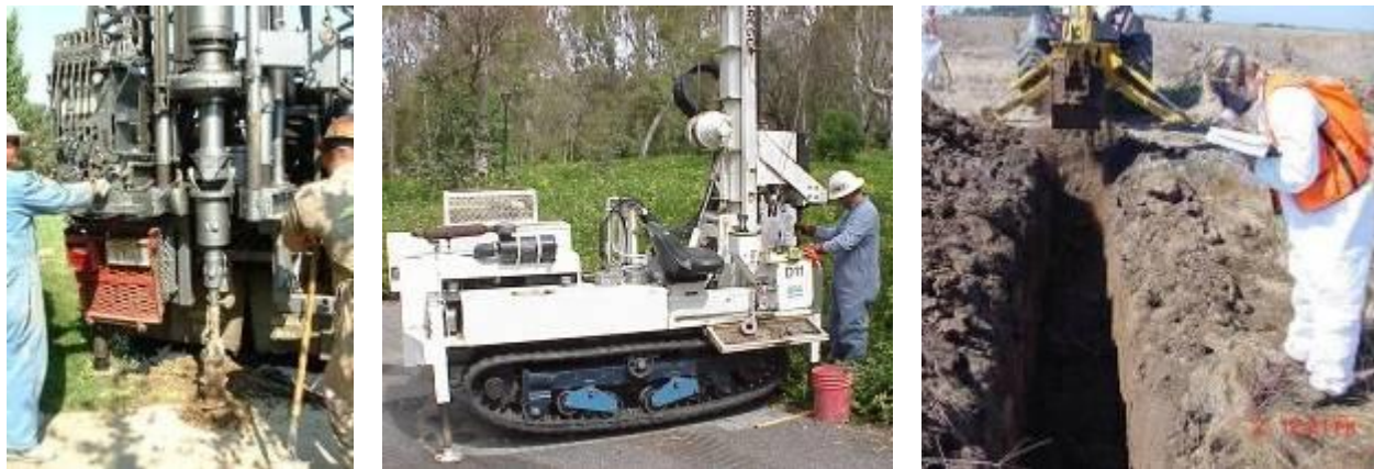
Figure 12: Intrusive or Invasive Investigation may include: drilling, direct push (Geoprobe) and trenching
