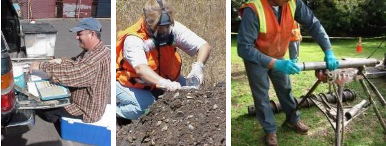
Figure 17: Sampling and analysis of waste and soil within landfill to determine physical and chemical characteristics; Removal of sampling core from split-spoon sampling tool used in a hollow stem auger drill rig
