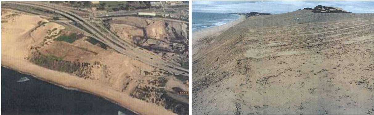
Figure 3: Photograph of Sand City dump before remediation; note front slope of dump toward public beach which contained rubbish, cans, glass and burned materials; photograph on the right shows completed final grades and wastes removed from front slope.
