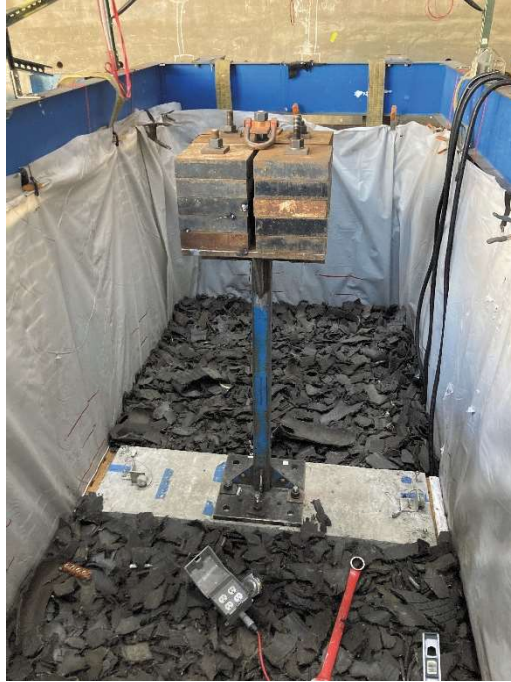
Figure 6.13 Placement of footing, SDOF system and surrounding TDA.
