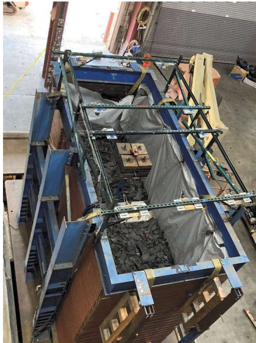
Figure 6.14 Top view of test specimen built on shake table after placement of steel frames for instrumentation support.
