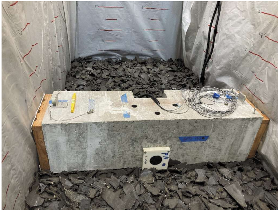
Figure 6.12 Placement of footing on top of TDA.
