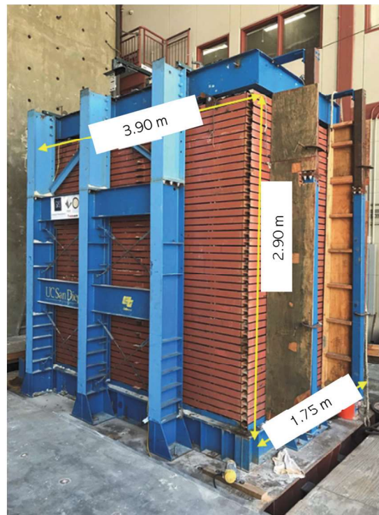
Figure 6.3 Laminar shear box on top of the shake table in the UCSD Powell Laboratory.
