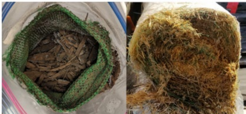
Figure 1B: The filling of a sample of SW (left) and CFS (right) collected after the Camp Fire. Photo credits: John Machado.
