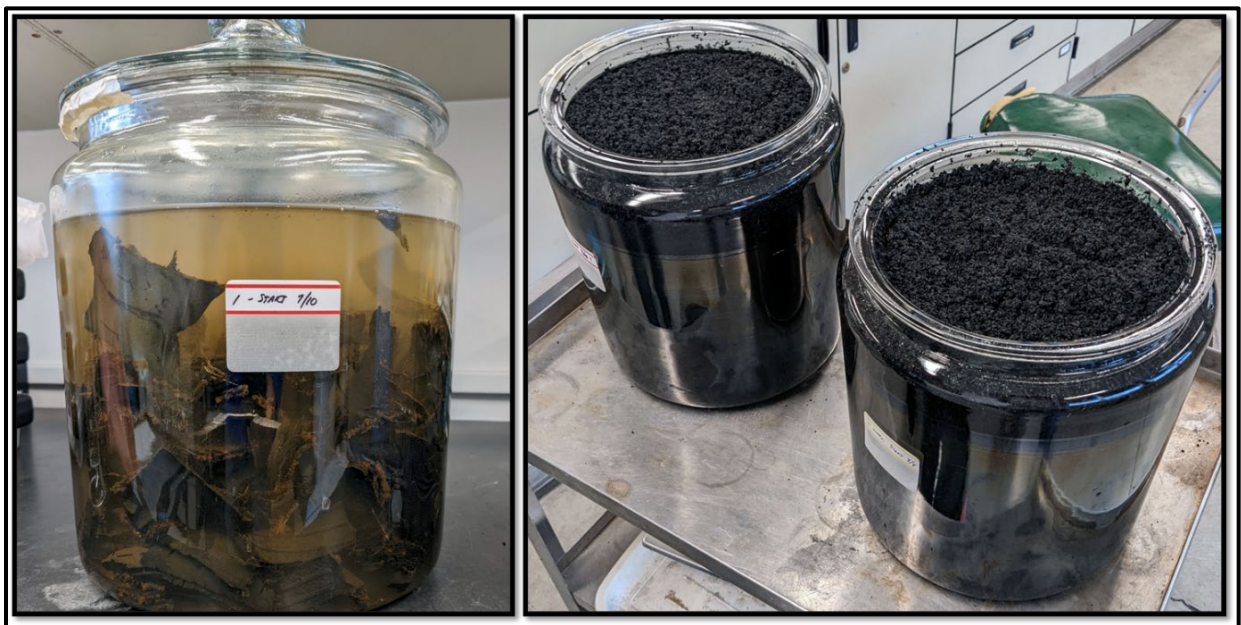
Figure 2. Soaking TDA-A (left) and tire rubber crumb (right).
