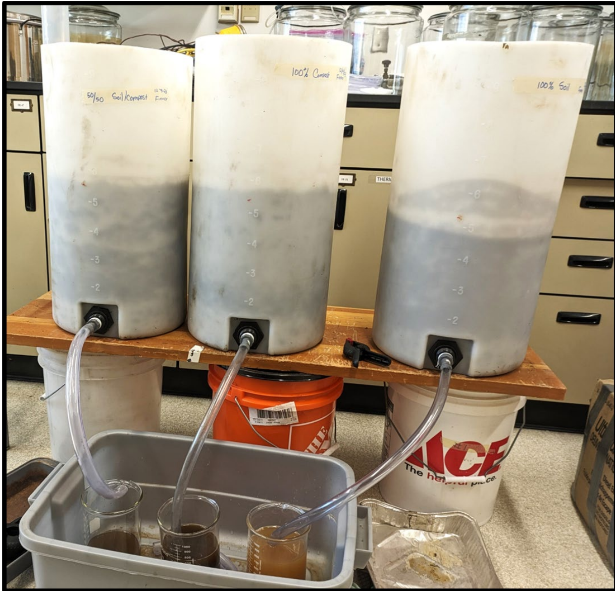
Figure 4. 12-inch diameter HDPE filtration columns.
