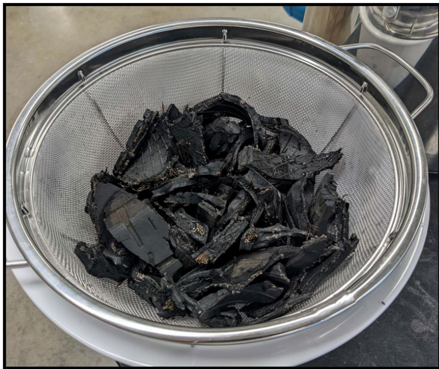
Figure 3. Preparing to sprinkle water over TDA-A.
