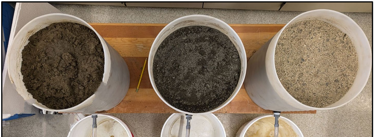
Figure 6. Construction fill media used for filtration; from left high-clay fill soil, river sand, beach sand.
