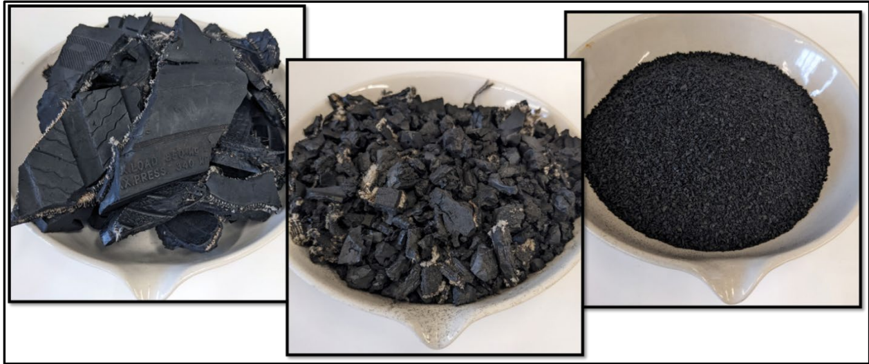
Figure 1. Source materials used for producing leachate containing 6PPD-Q: from left TDA-A, tire rubber mulch, tire crumb.
