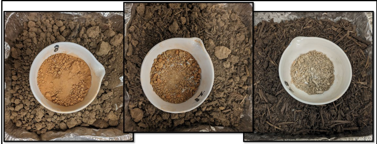
Figure 5. Filtration media (with nonvolatile portion in the dish for comparison) for 9-inch depth test; from left topsoil, topsoil/compost mix, compost.
