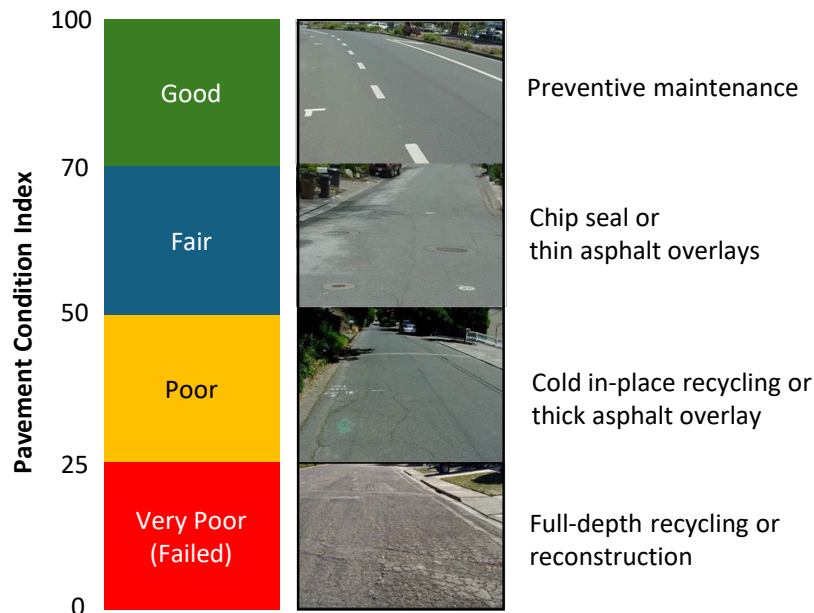
Figure 3. Example PCI thresholds, conditions, and typical treatments (source: NCE)
