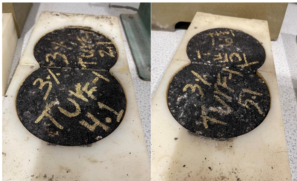
Figure 16. Samples for Rutting Test
