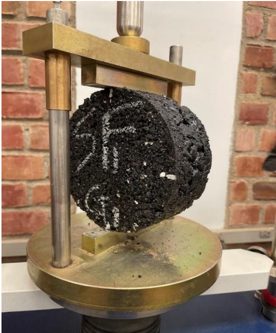
a) Sample before IDEAL-CT Test
