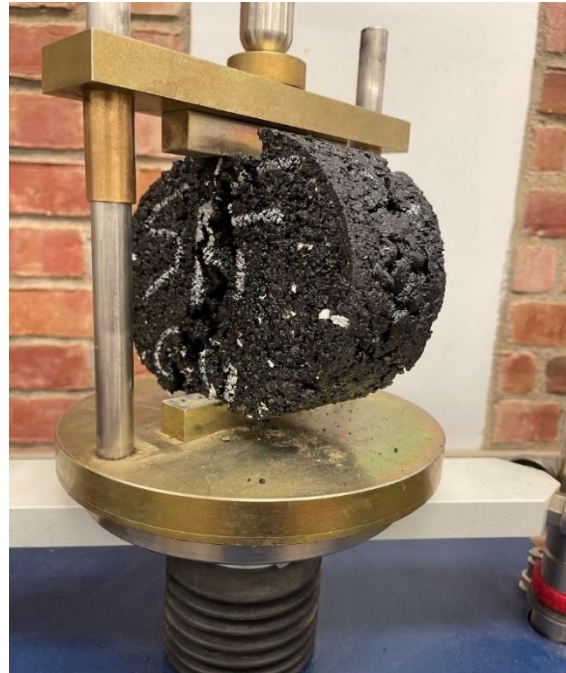
b) Sample after IDEAL-CT Test
