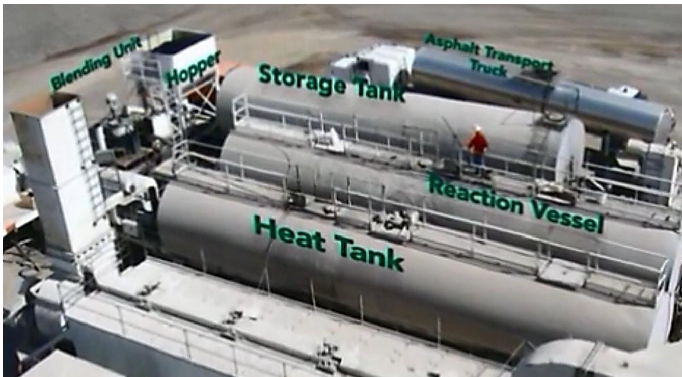
Figure 1. Mobilized equipment needed for Asphalt-Rubber Hot Mix
