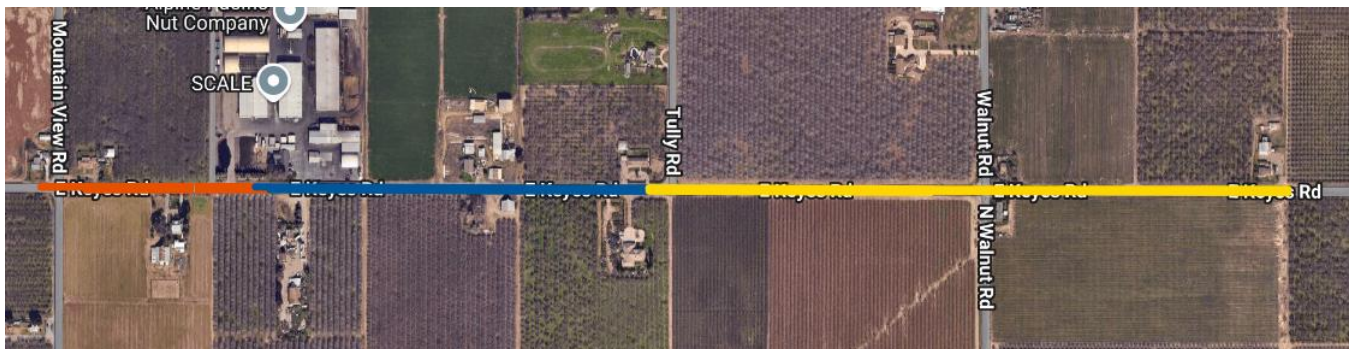
Figure 3. Material placement limits – Orange represents SmartMIX™, blue represents PelletPAVE-TR, and yellow represents the HMA control
