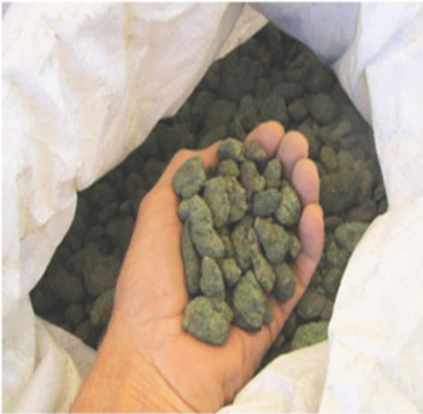
Figure 14. PelletPAVE-TR sampled from bulk delivery bag
