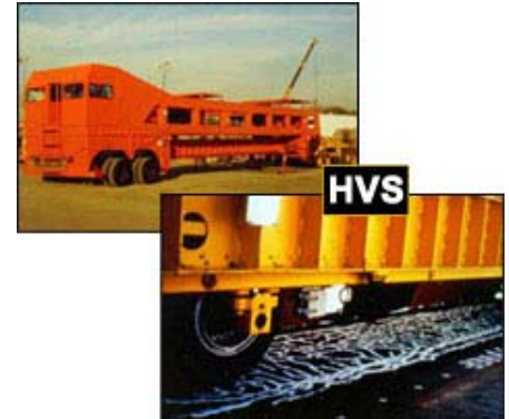
Heavy Vehicle Simulator used for the 1992 Caltrans research
