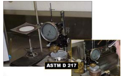
Cone Penetration Test
