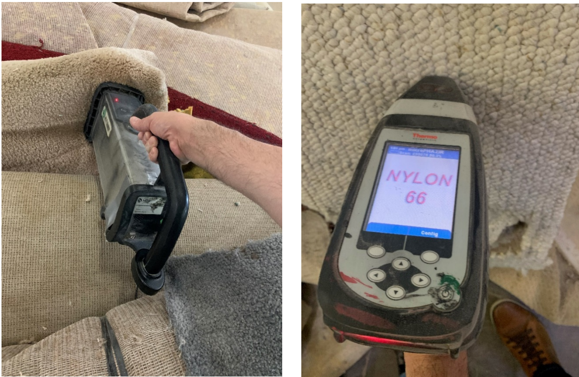
Figure 4-1. Carpet Fiber Identification Devices Indicating that Carpet is Nylon 6,6
