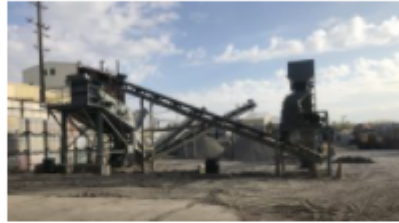
Aggregate crushing and screening equipment at Visions Environmental's plant in Oroville
