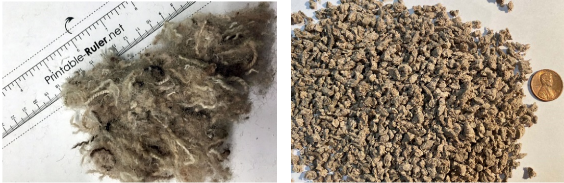
PET fiber (left) and PET agglomerated pellets (right).
