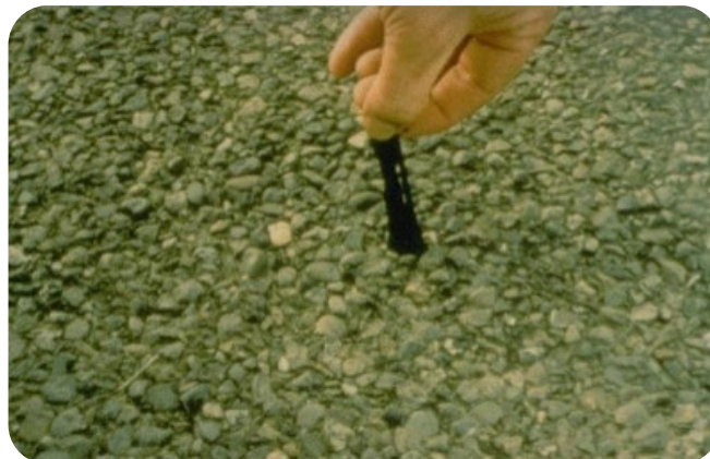
Figure 18. Pull test of chip seal aggregate and asphalt rubber binder.
