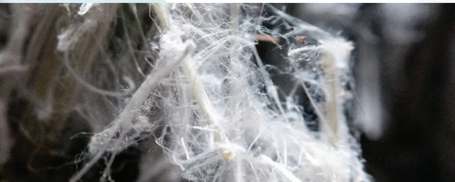
Asbestos in insulation is often white, layered, and has curly fibers.
