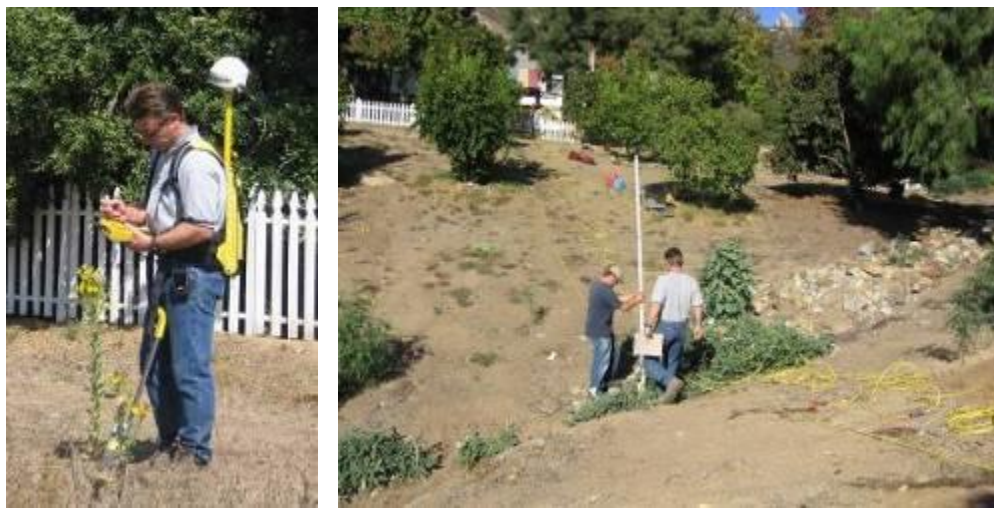
Figure 10: Using Trimble GPS Surveying Equipment to locate Geophysical Survey Results; Resistivity Survey on a Burn Dump in San Diego County
