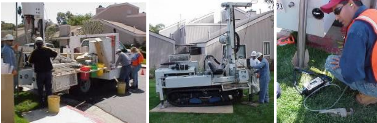
Figure 34: Two types of hydraulic direct push rigs were used to define the extents of waste; combustible gas instruments were used to obtain gas measurements in the direct push boring; gas samples were collected in Summa Cannisters for laboratory analysis
