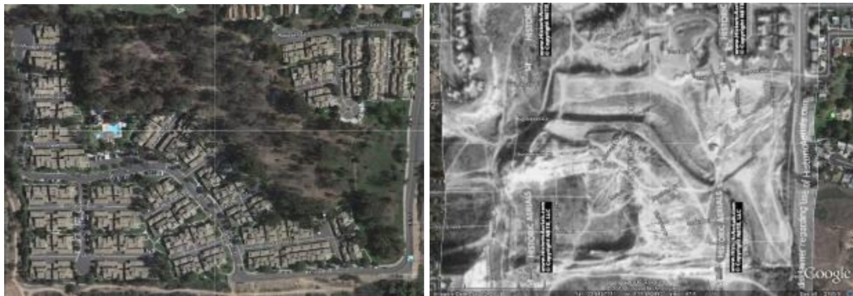
Figure 33: Newport Terrace Condominium Aerial Image. Park area is the former City of Newport Dump No. 1; Condominiums were constructed adjacent to and on top of the former disposal site. The condominiums shown in the lower left portion of the aerial image were constructed on a disposal fill area that was covered with 10-15 feet of
