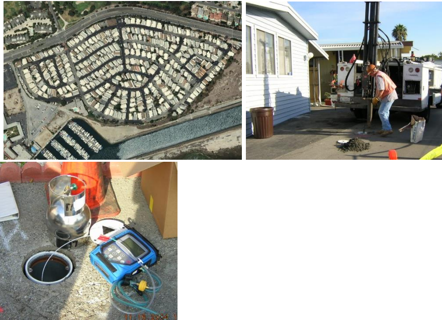
Figure 10: Aerial Photo of Long Beach Mobile Home Park; Direct-Push Equipment; Gas Screening & Sampling
