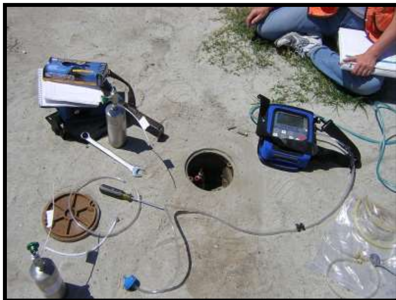
Figure 44: Landfill gas sampling and screening using Summa canisters and a GEM 2000
