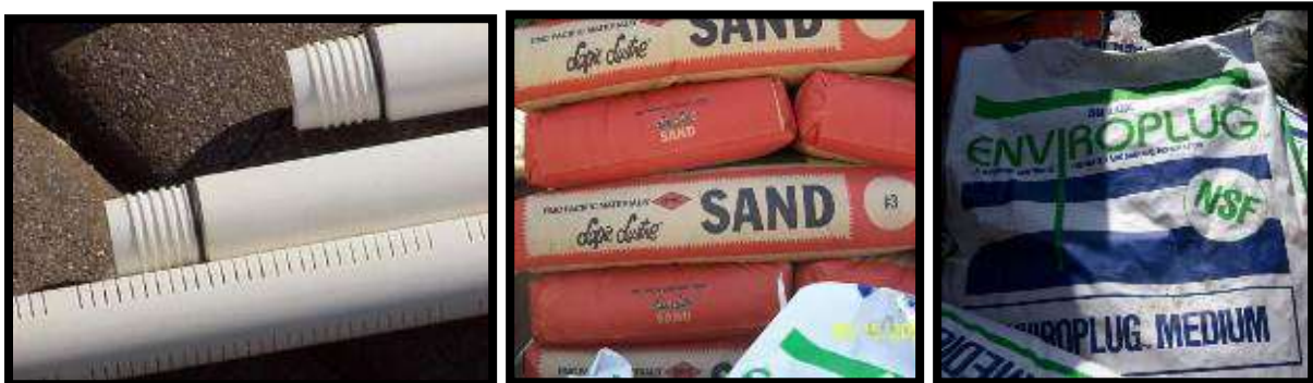
Figure 23: Landfill gas monitoring well materials: 1) monitoring probe: schedule 80 PVC machine-slotted pipe in 8-foot threaded sections; 2) screen well pack: Monterey sand or equivalent, 3) well bore seal: bentonite (pellets)
