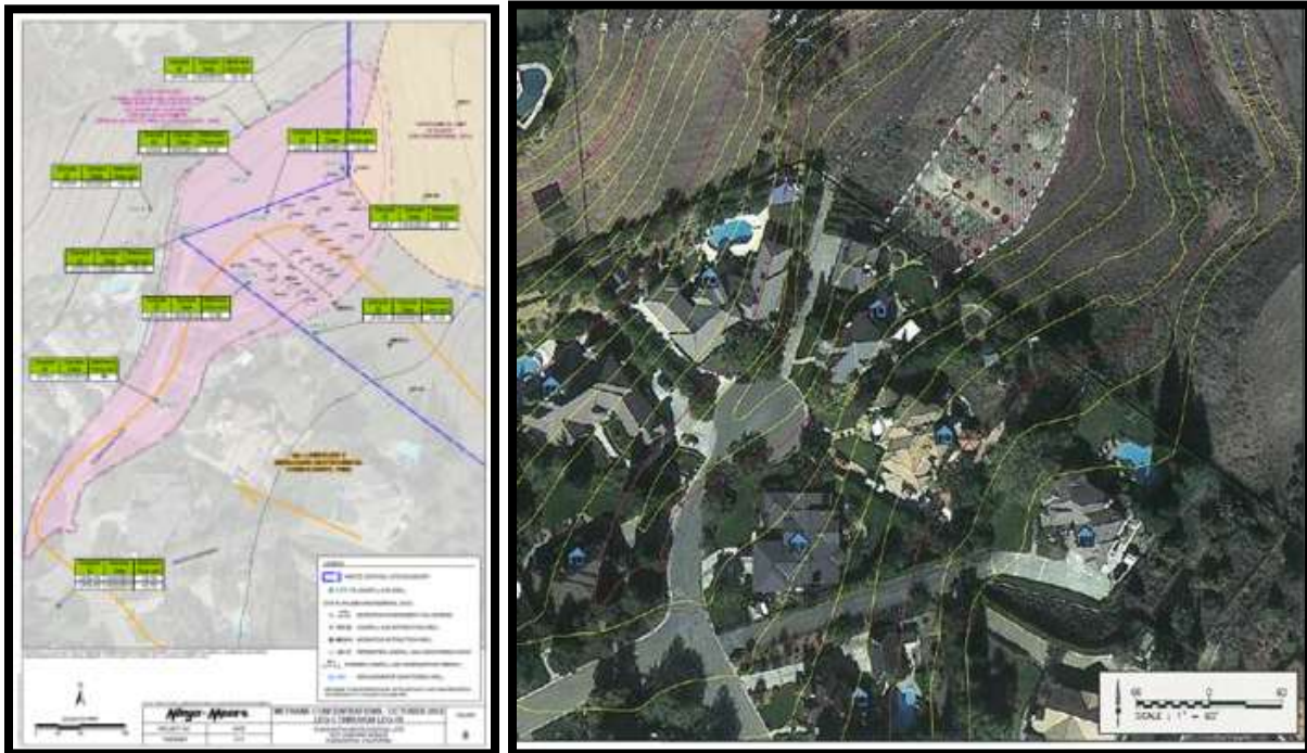
Figure 54: Investigation map showing CalRecycle gas monitoring well locations and landfill gas concentrations (note LFG-2 at 18 percent); EBA topographic map showing homes in Gray Fox Circle (LFG-2)
