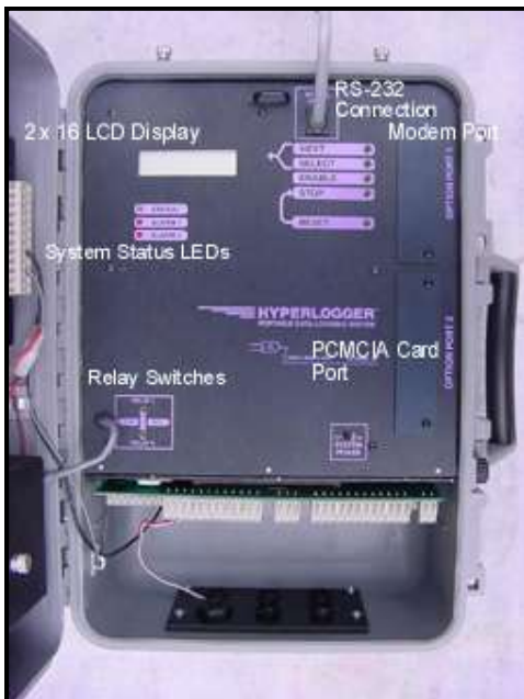
Figure 36: The Hyperlogger is a data-logging system (by Logic Beach)
