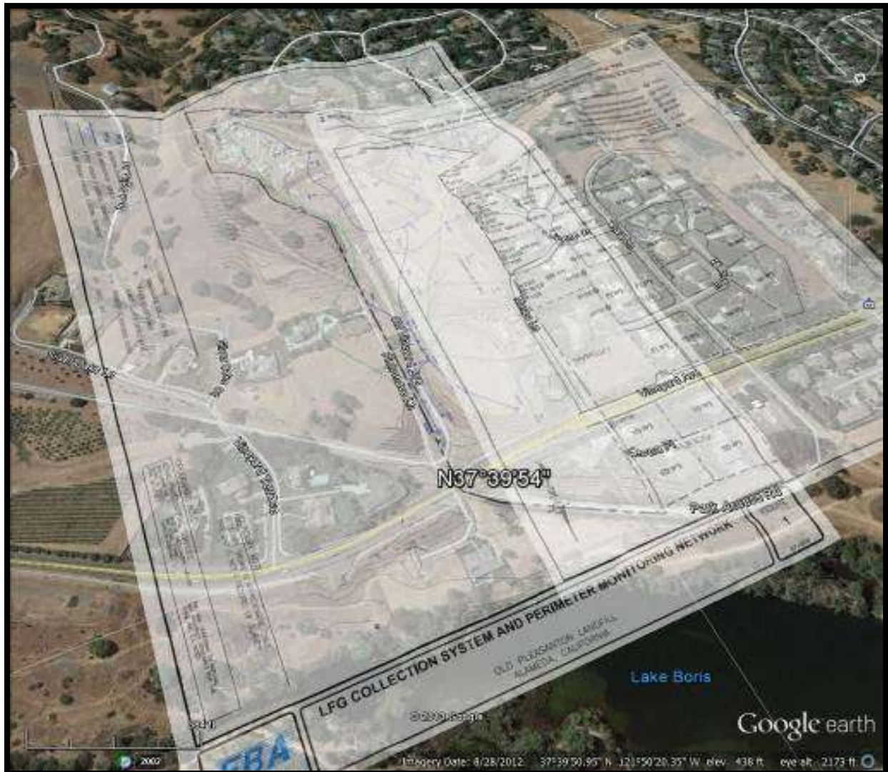
Figure 53: Landfill gas collection and perimeter monitoring plans overlaid on a Google Earth aerial image of the Old Pleasanton Landfill provide a 3-D perspective of the site and layout of the landfill gas collection system and perimeter monitoring network. Note: The drawing overlay on the right is the landfill gas migration system installed in the Delco Property development west of the landfill. Landfill gas migration was detected in off-site monitoring wells in the subdivision south of the site (located at top of figure).
