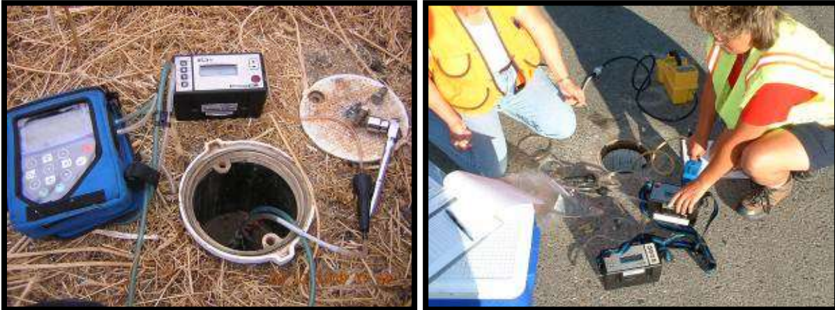
Figure 29: Landfill gas monitoring equipment; note that 2 different instruments are used to verify field measurements (GEM-2000, RKI Eagle and GMI 442) for field quality assurance/control.
