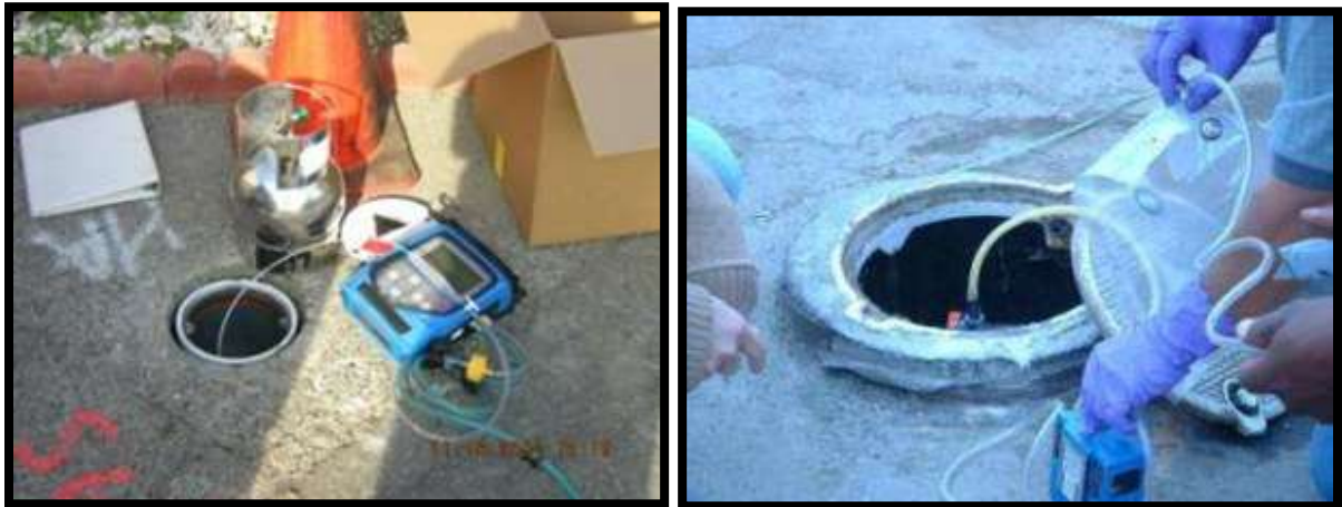
Figure 32: Landfill gas sampling – using Summa canisters and Tedlar bags
