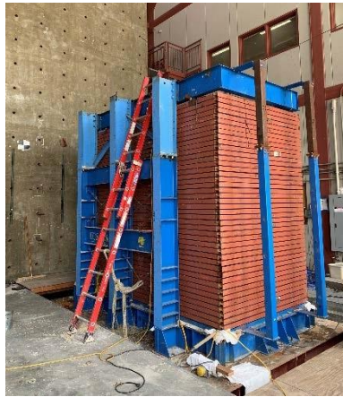
Figure 1: Picture of large-scale laminar container available at UCSD
