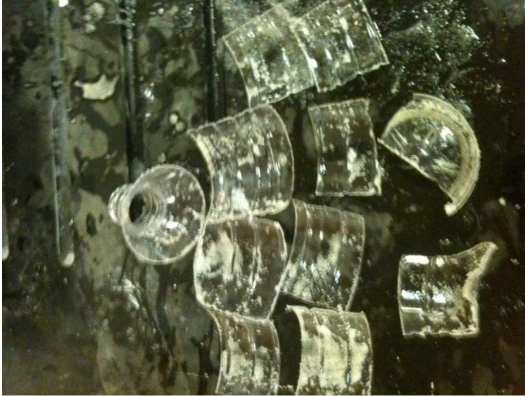
Figure 17. PLA sample after 365 days in the water bath disintegration test.
