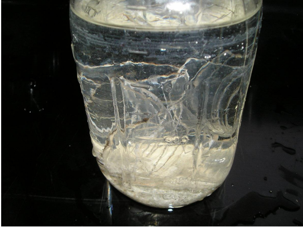
Figure 16. PLA sample at the start of the water bath disintegration test.
