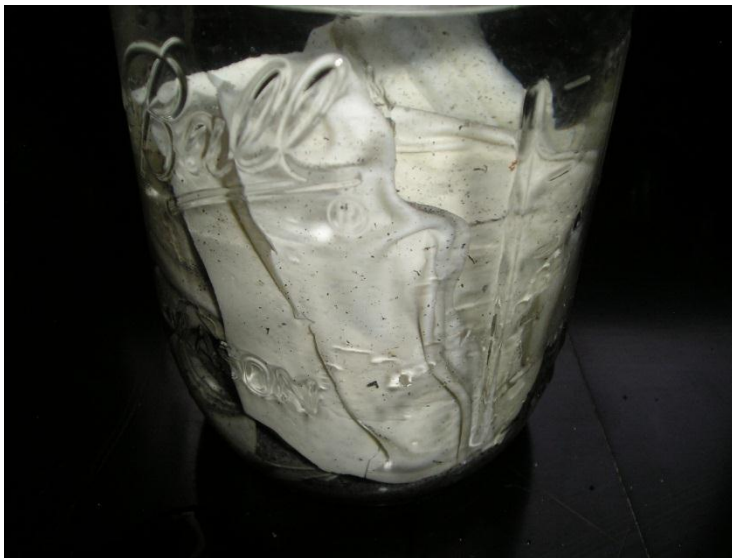
Figure 13. PHBV sample with water bath disintegration tests after 180 days.
