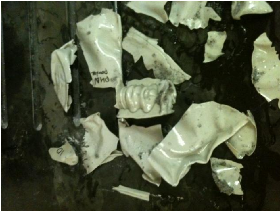
Figure 15. PHBV sample after 365 days in the water bath disintegration test.
