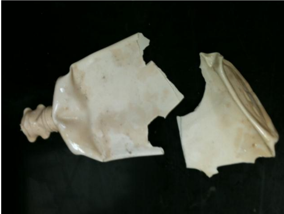
Figure 9. PHBV disintegration evaluation after 365 days at 30°C.
