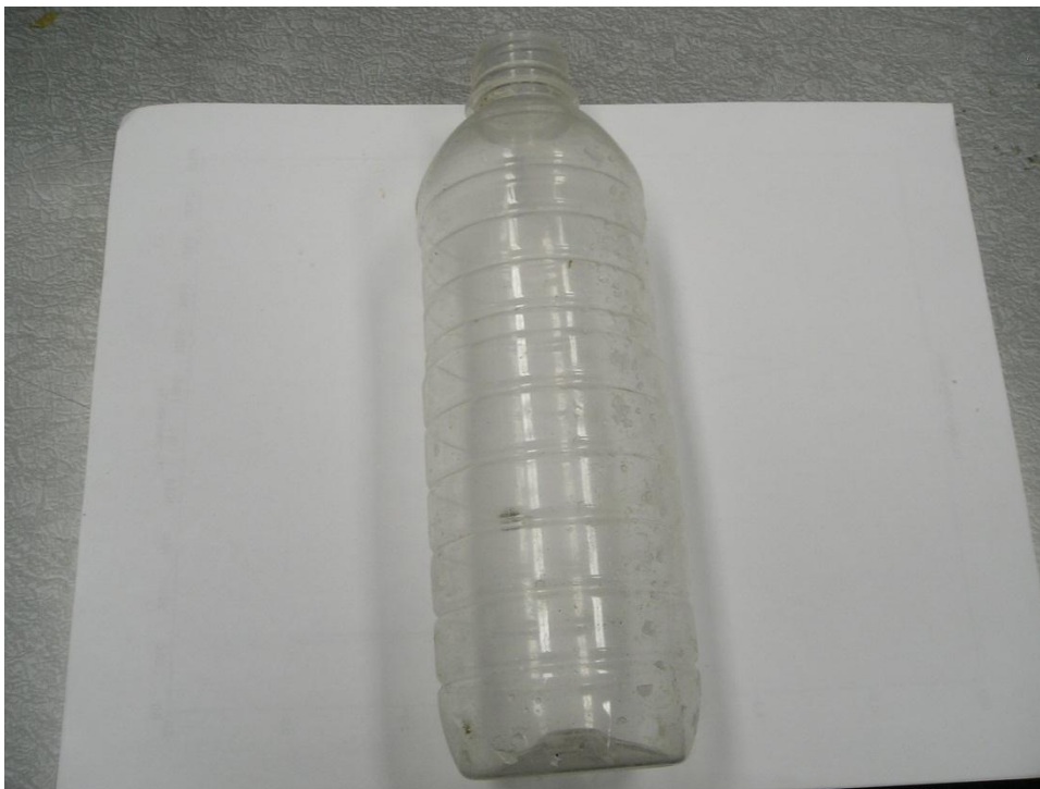
Figure 10. PLA disintegration evaluation after 144 days at 30°C.
