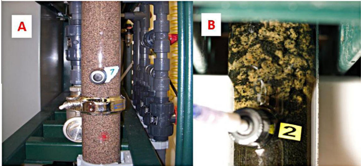
Figure 5.11: Growth of biomass suspended in the FBR column. Growth of pink-pigmented Type I methanotrophs after 47 days is shown at left. Growth of tan-pigmented Type II methanotrophs under selective conditions after 252 days is shown at right.
