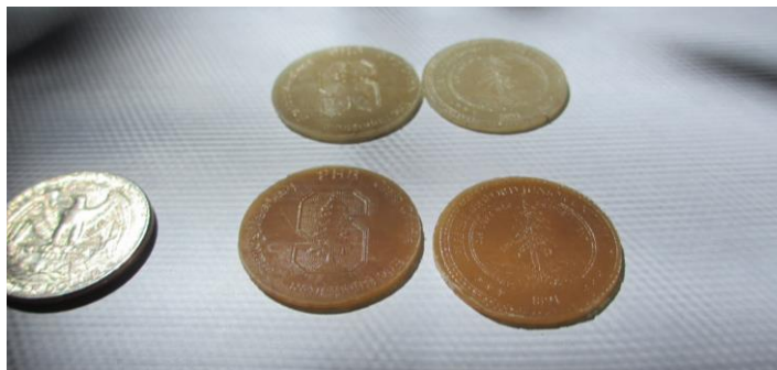
Figure 6.1: Plastic coins extracted using a combined SDS and hypochlorite extraction protocol. The top two coins are commercial PHBV; the lower coins are PHB from methanotroph biomass.
