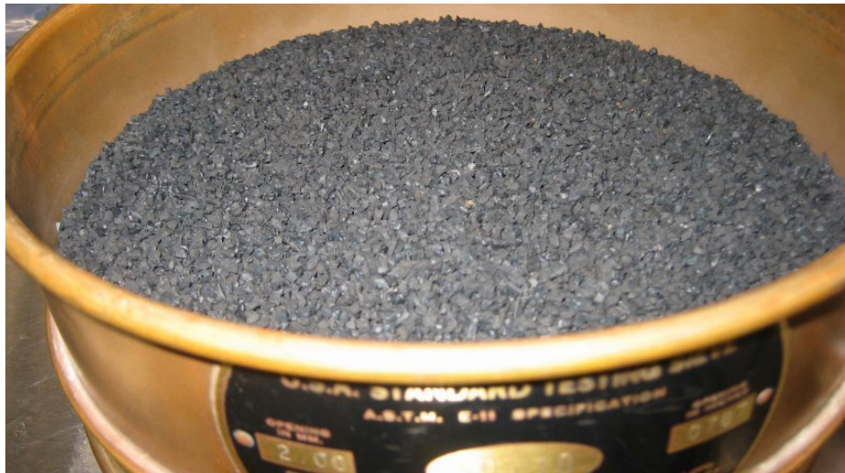
Figure 1: A representative sample of passenger tire crumb rubber that is less than 2 micrometers in diameter.
