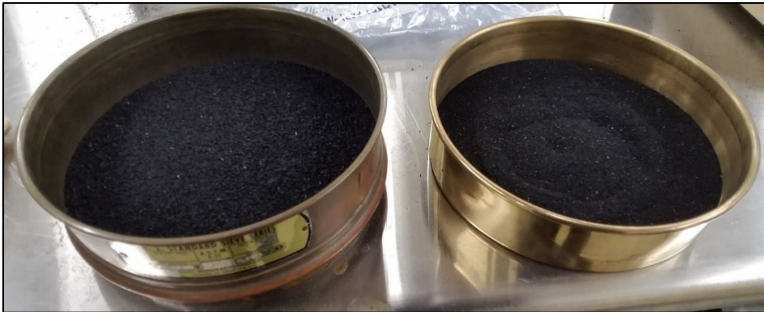
Figure 2: Two size classes of passenger tire crumb rubber were selected as greater than 0.5 mm (large, on left) and less than 0.5 mm (small, on right).
