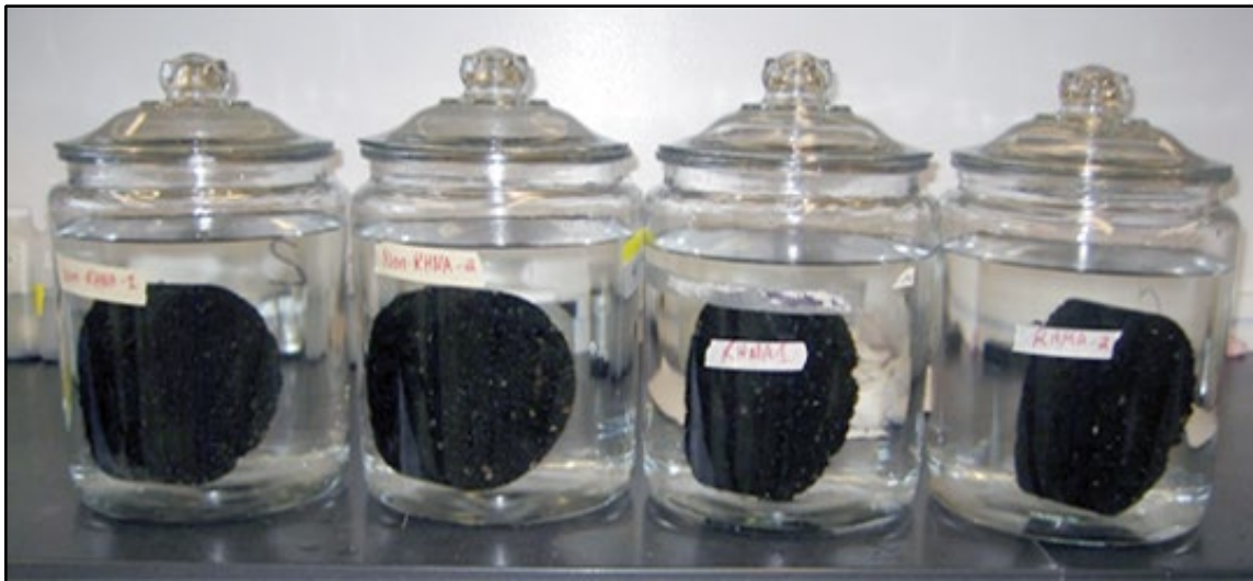
Figure 4: Four identical RHMA pavement cores were each placed in distilled water to determine the zinc leaching rate over time.
