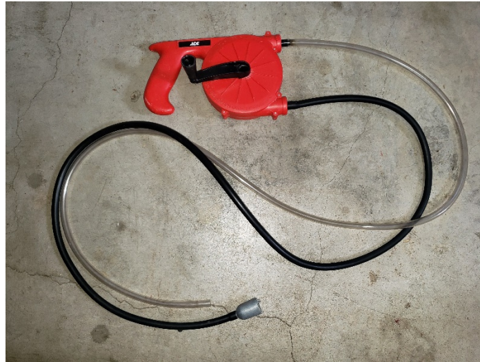
Figure 7: The rotary hand pump used to collect stormwater runoff samples from pavement.
