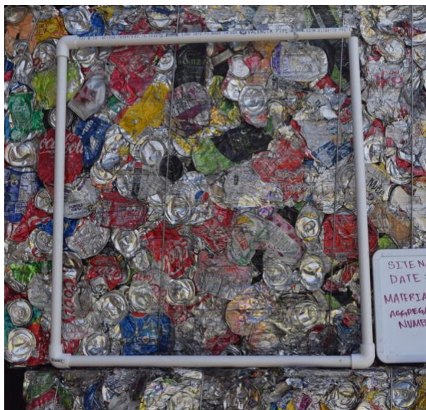
Figure 3. A quadrat used for measured photos of bales and other outflows.
