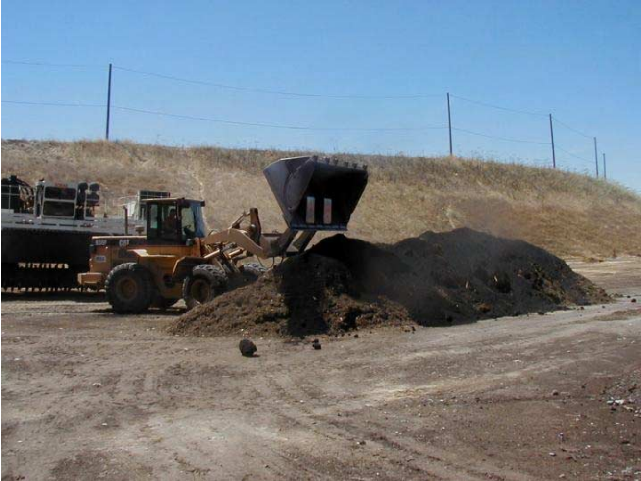
Photograph 1: Wood ash being incorporated into compost at Lionudakis Wood and Green Waste Recycling in Sacramento.
