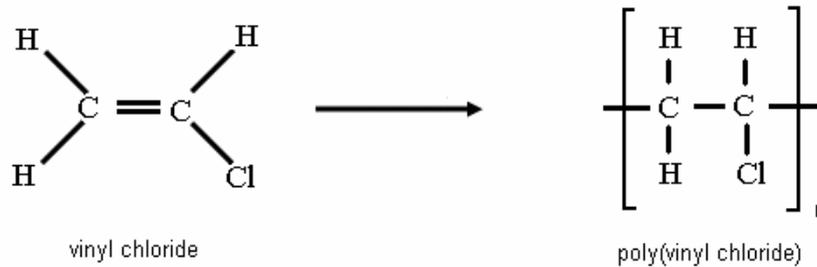
Figure 1: Structure of vinyl chloride monomer and polymer of polyvinyl chloride.
