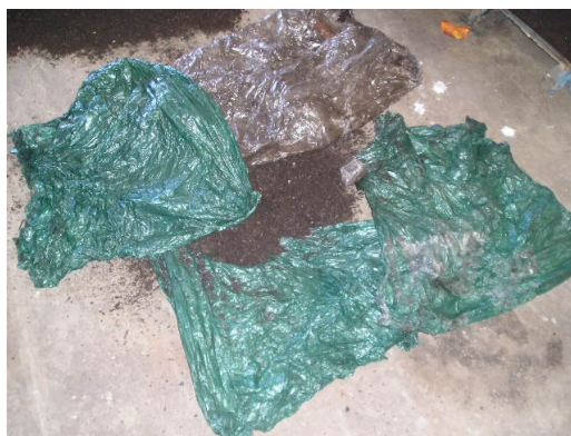
Oxodegradable and UV degradable (180 days)
