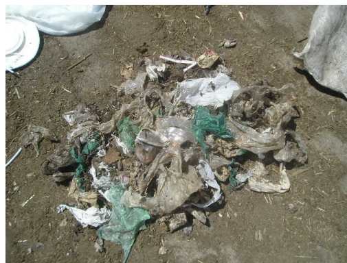
Oxodegradable, UV degradable, LDPE bag, and debris (170 days)
